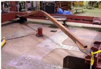
(a) Buckled out poor nonlinear behavior of conventional braces
